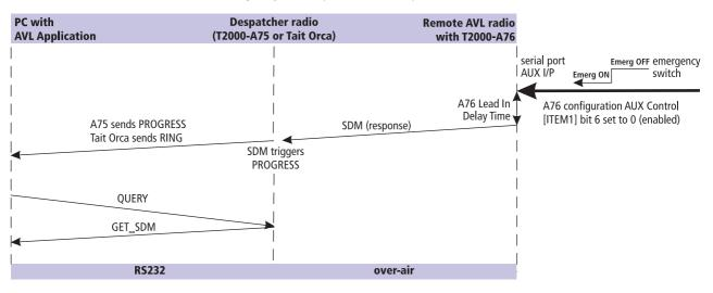
The operation of Emergency mode is controlled by the following configuration items - refer to the A76 Configuration section:
