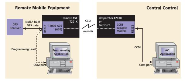
The despatcher radios uses the Tait CCDI (Computer Controlled Data Interface) over-air command protocol to communicate with the remote radio. CCDI commands containing short data massages (SDMs) are sent to the remote radio by the PC AVL application. Each SDM contains a command which tells the remote radio to one of the following:
